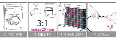
To use SuperClean<sup>™</sup> as a heavy duty, foaming cleaner for aluminium-finned, air-cooled condensers, dilute with 3 parts water. Using a low pressure sprayer, spray between the fins – starting at the bottom in one corner and progressing methodically across and up. Cleaning is more effective if coil is still warm. In minutes a heavy foam will form, forcing contamination outwards. Foam and contamination must then be rinsed away thoroughly with fresh water.
