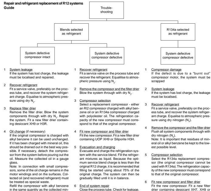
Refill the compressor with alkyl benzene in the same quantity as the collected mineral oil. Refit the compressor into the system.
