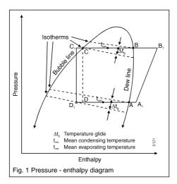
The blends in table 1 are non-azeotropes. Therefore the composition changes during evaporation and condensation. This leads to temperature changes at constant pressure.
