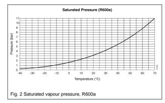
Both solutions presuppose that the vapour pressure in the system is higher than 1 bar. Fig. 2 shows the saturated vapour pressure as a function of the temperature.
