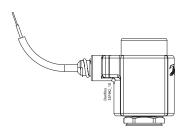
To ensure correct sealing between coil and valve mount the coil in the proper position and make sure that the coil is fully clicked on to the valve.
